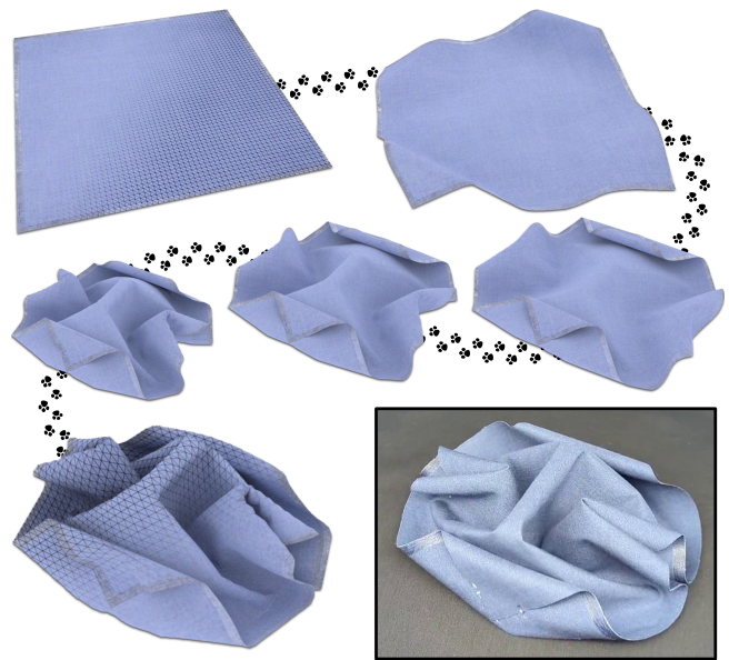
Figure 1: Our method automatically generates a diverse set of folding patterns using strain-space modes. Here we show a particular folding transformation for a square sheet of fabric and its physical prototype (bottom right).
